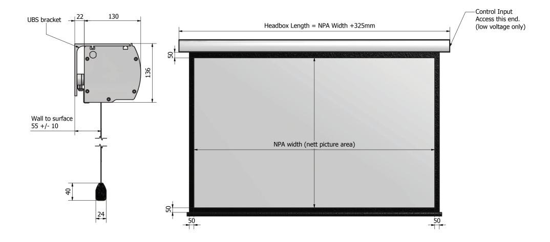
Manufacturing tolerance +/-5mm on headbox and slatrod All dimensions are in (mm) If installed in ceiling always allow for removal for servicing.
